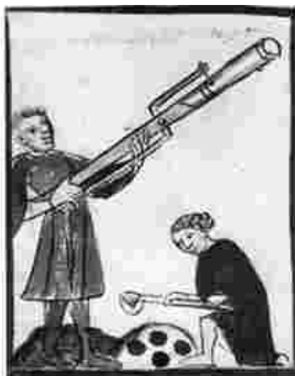
First illustration of a serpentinelock. The other figure is casting bullets. From a manuscript of 1411 (Codex Vindobana 3069, Austrian National Library, Vienna)
