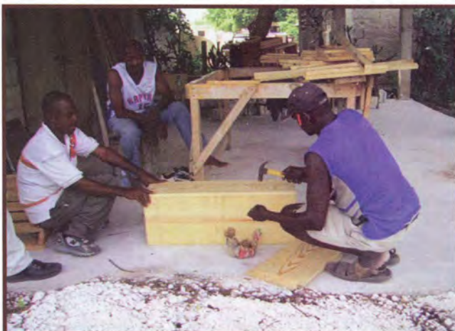
At the shop of the Apiculture Association of Aquin local carpenters constructed a Kenya top bar hive using hand tools.
