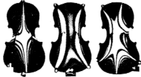
First, second, and third modal vibrations of violin top plates under hologram interferometry, left to right, at 80, 147 and 222 Hz.
