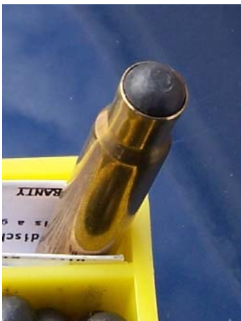
Sized buck shot pressed into the mouth of the Game Getter modified cartridge.
