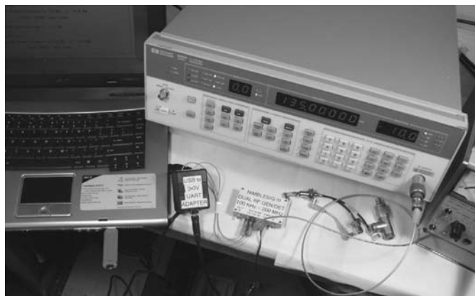
The NimbleSig III connection daisy chain shows the parallel port JTAG interface connected to the 20 pin side of the cross-connection board and the NimbleSig III 10 pin JTAG programming cable connected to the 10 pin side.
