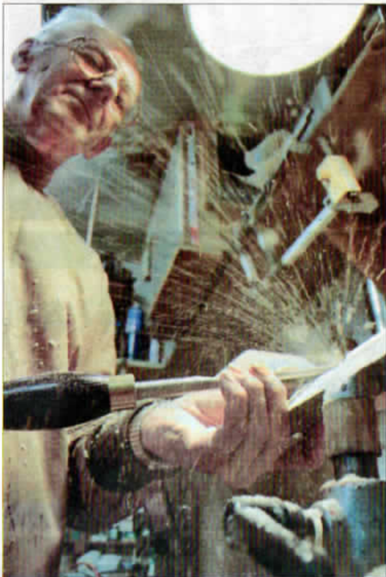
Using his lathe, Colin Delory fashions ball and cup toys from wood.
