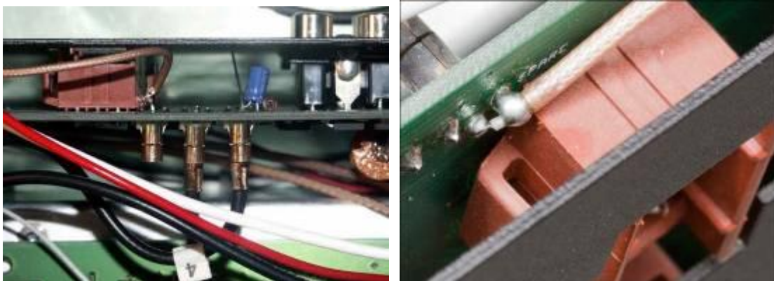
Figure A-5: Spare jack connection (Photo at right Courtesy of Roberto Barrios, EB4EQA)
