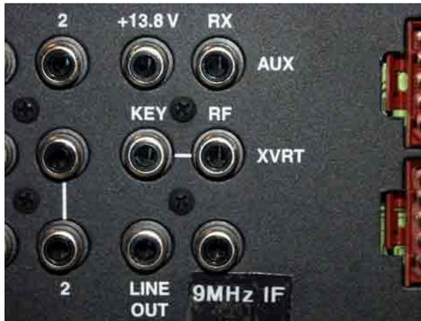
Figure 11: Rear Connector on Orion 565
