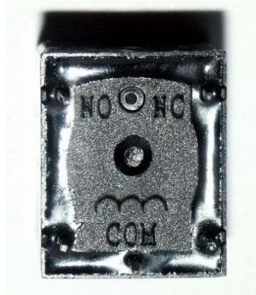
Relay – Coil and common connection are at the bottom of the figure
