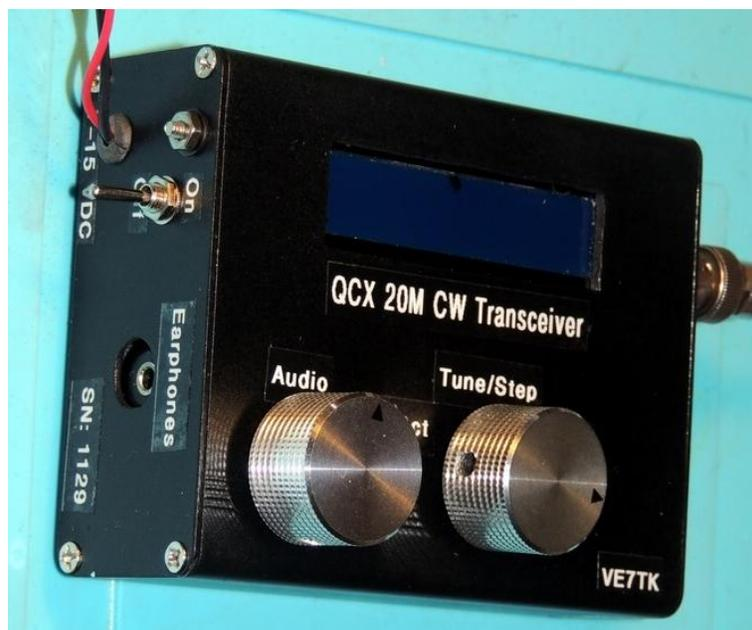
QCX – Showing On/Off switch and LM7805 heatsink attachment
